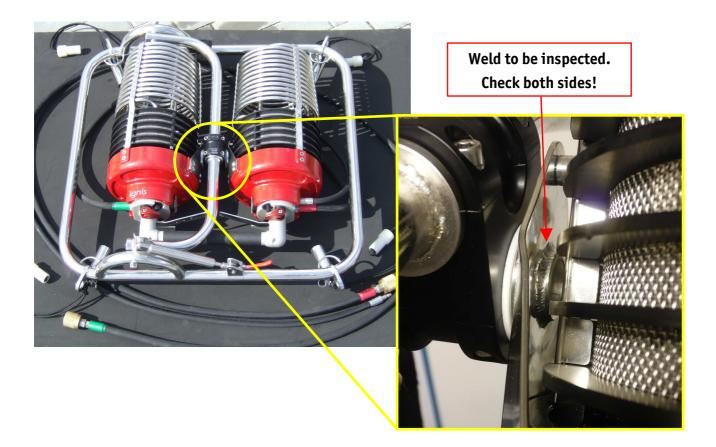
Check the weld along its entire length for possible cracks. Use a flashlight to see it well and try to move the burner in the hinge. In case the weld is damaged the burner unit is likely deflected from its correct position and the blast valve lever is not exactly above the handle.
